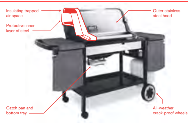
Double-walled hood construction
