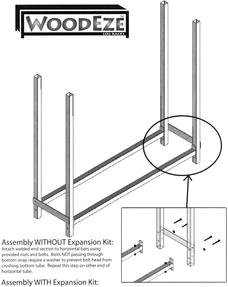
Attach welded end section to horizontal bars using provided nuts and bolts. Bolts NOT passing through bottom strap require a washer to prevent bolt head from crushing bottom tube. Do this on one of the welded end sections then follow instructions in the expansion kit.
