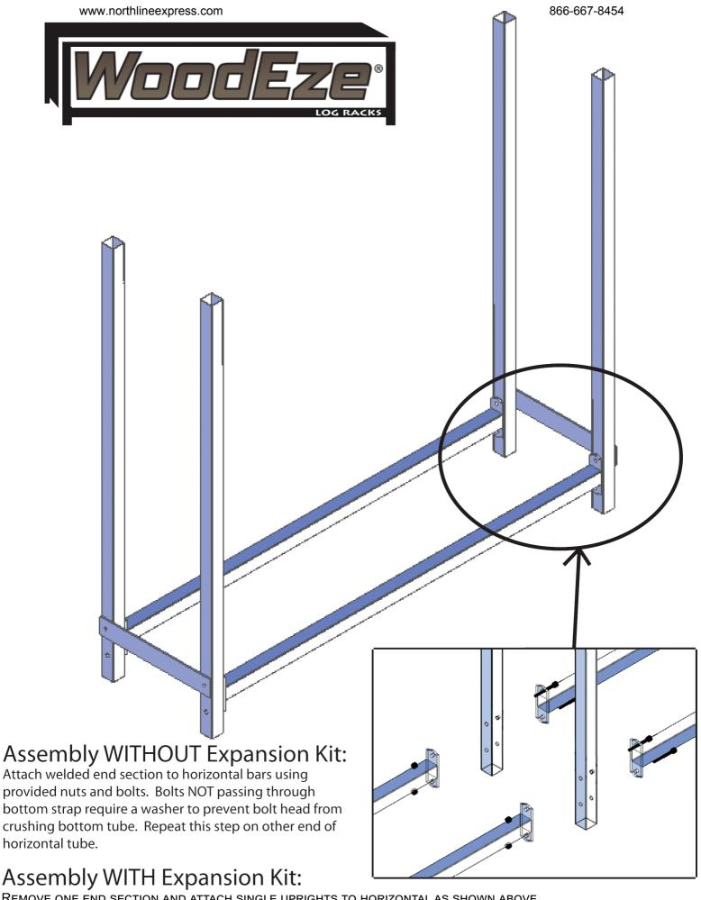
REMOVE ONE END SECTION AND ATTACH SINGLE UPRIGHTS TO HORIZONTAL AS SHOWN ABOVE. REATTACH END SECTION TO HORIZONTAL ENDS.
